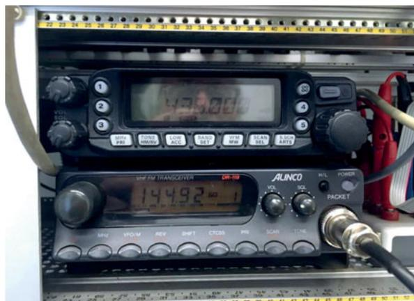
Transceiver Oben: Packet-Radio OE9XFR 70cm 9k6
